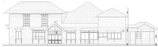
[Fig. 6] Elevation drawing created by tracing the 3D model, Former Kon's residence
